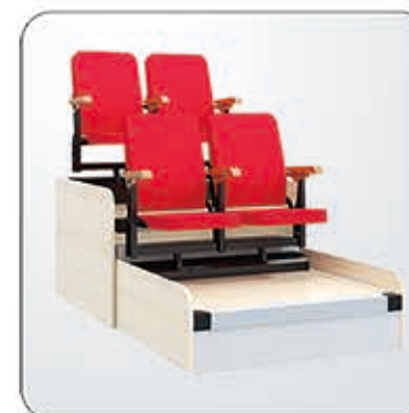
SJ-A036 后置带扶手软包椅 SJ-A036 Rear upholstery chair with armrest Width:900mm Height:310mm Seat Center Distance:500mm Seat Type:Rear-Back Upholstery Chair with Armrest Drive Mode: Manual or Electric Seat Flip Mode: Manual or Automatic
